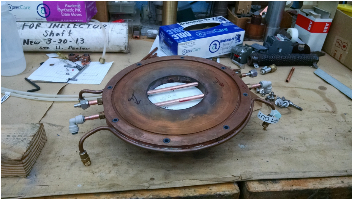
FIG. 2. The new cooling line installed in the magnetic filter region of the H^- source. The north poles of the permanent magnets are aligned perpendicular to the path of the extracted beam as shown above.
